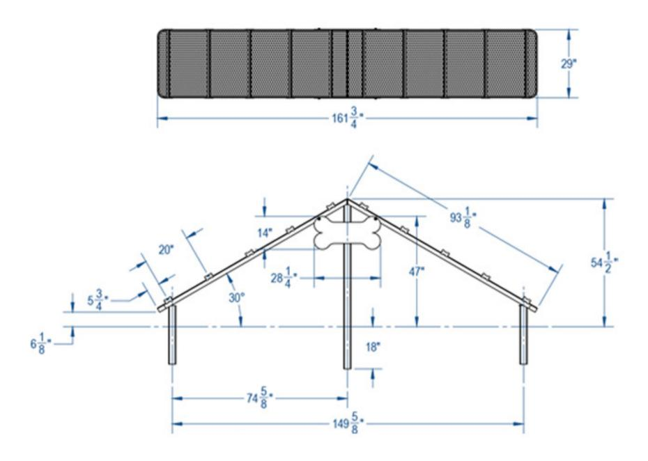
Dog Climb Deck Material: Outer frame is made from 3/4" x 2" rolled form angle iron.
