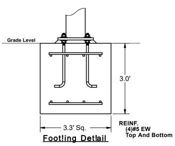
\*Footing design based on 1500 PSF soil bearing pressure.
