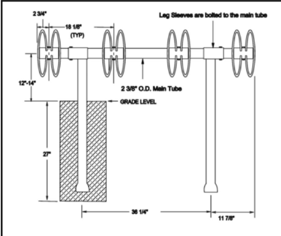
Loops are welded to sleeves and sleeves are bolted to the main 2 3/8" O.D. tube
