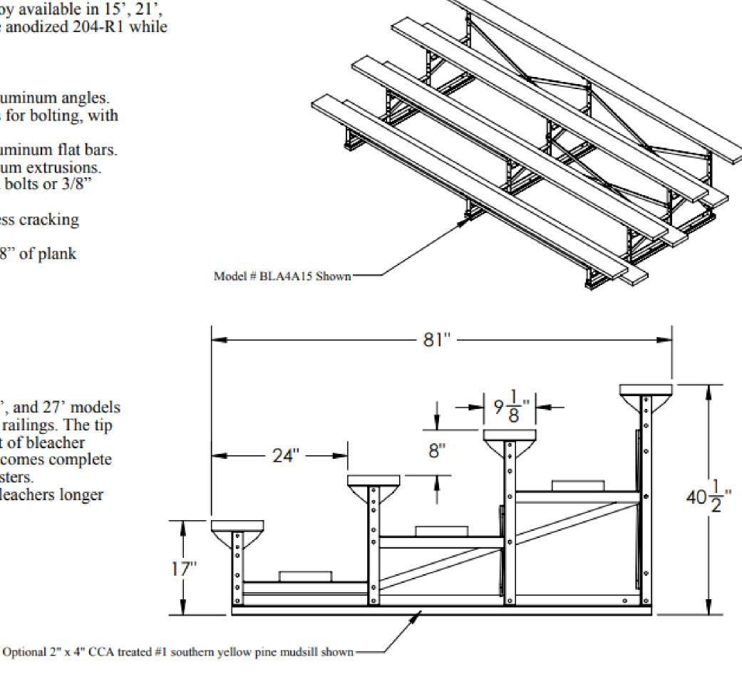
THESE BLEACHERS & FRAMES ARE DESIGNED AND TESTED TO BE IN ACCORDANCE WITH FEDERAL SPEC. # RR-B-425-C AND THE 2006 IBC WITH THE EXCEPTION OF THE REQUIREMENT FOR AN AISLE.
