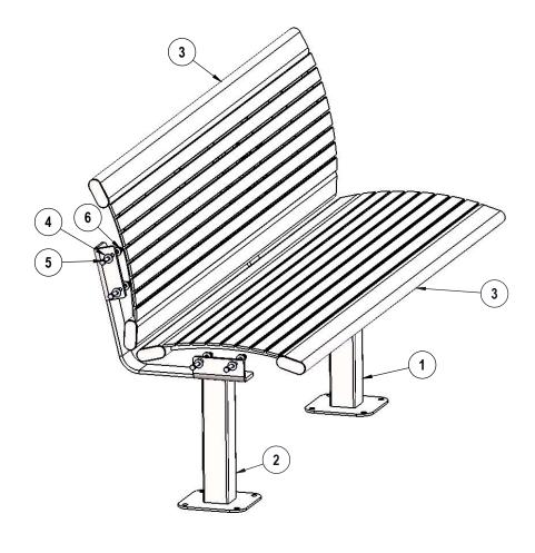
Recommended Surface Mount Hardware: 3/8" x 3-1/2" Concrete Expansion Anchor Bolts (Not Included)
