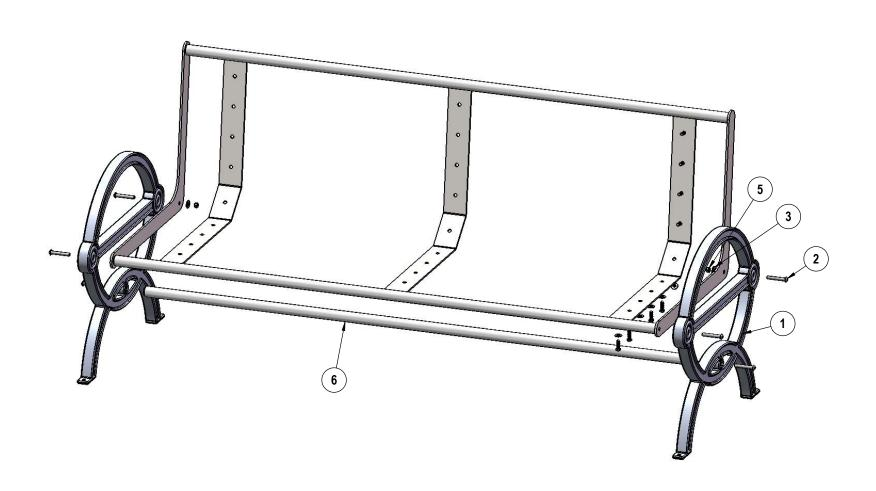
Attach the Recycled Seat Support and support bar to the Cast End Frames using the specified hardware.
