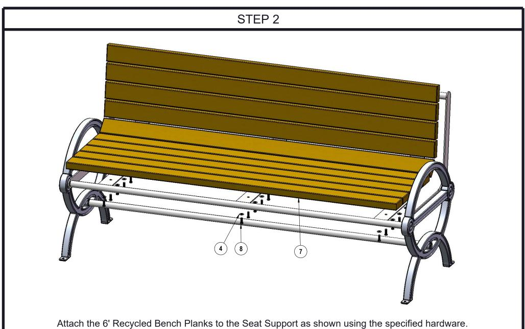
Warning: Over tightening of the Lag Bolts may result in cracking and/or stripping out of the Planks.
