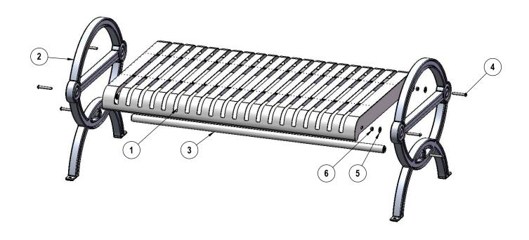
Optional Surface Mount Hardware: 3/8" x 3-1/2" Concrete Expansion Anchor Bolts (Not Included)
